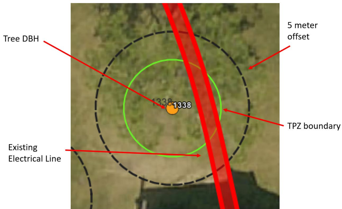
Figure 3. Example of GIS Utility Overlay for Identifying Conflicts.
