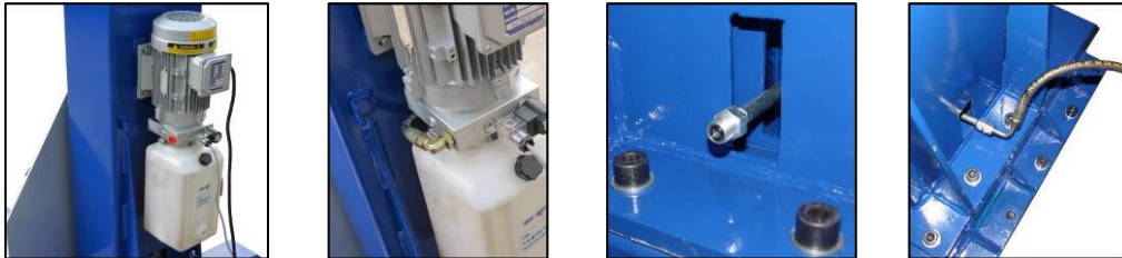
Fig. 7-A, B, C, D pump & hose
